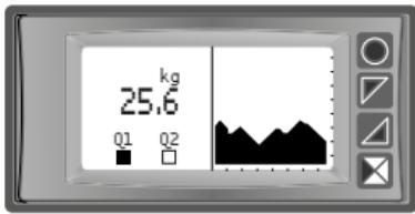
This page displays the process, the relays status and a graph representing the process trend.
