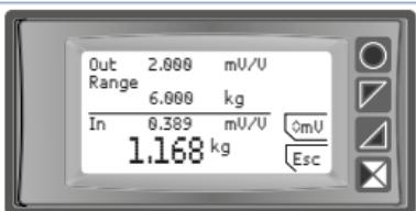
Press “**ØmV**” to go back to setting of mV/V ratio.
