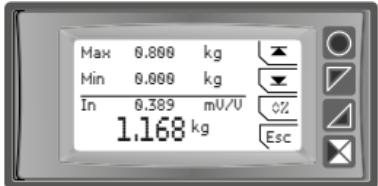
Press “**↙**” to calibrate lower limit and “**↗**” to for the upper limit. Press “**Ø%**” to go back to calibration percentage.
