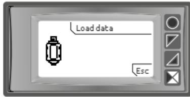
The user can either "Load data" load the parameters from the memory card or "Esc" cancel the operation without modifying the current configuration.
