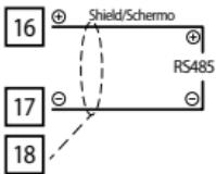
RS485 Modbus RTU communication
