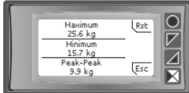
The STR56X is provided with a page for the visualization of peak values: max. peak, min. peak and peak-to-peak of analogue input. Keeping pressed "Rst" it is possible to reset the visualized values.
