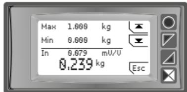
Press "↖" to calibrate lower limit and "↗" to calibrate the upper limit.
