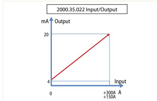
The 2000.35.022 has two dip-switches through which you can set the scale to 150 or 300A and select the monopolar or bipolar (see charts), the yellow led near the terminal will indicate the presence of the power supply. Any changes made by dip-switch required to switch off the power supply. It's a safety condition in order to prevent any manumission on the device.
