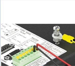
**Danger!** This device is only permitted to be supplied by a SELV / PELV (class 2) power supply or with safety extra-low voltage (SELV) in accordance with EN 60950.
