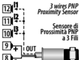
Example of connection of a 3-wires proximity sensor.
