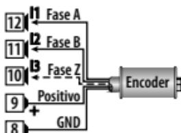
Example of connection of an encoder. The Z signal connection is optional. If the encoder absorbs more current than that supplied by the OUT 24V output according to the supply voltage, it may be necessary to supply the encoder with an external power supply.
