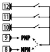
Example of connection of digital inputs in PNP and NPN mode.
