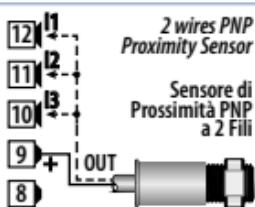
Example of connection of a 2-wires proximity sensor.
