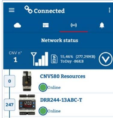
Third tab displays the status of the CNV580 and all the connected hardware resources. The top row is dedicated to the CNV status, and can be expanded to reveal additional info such as serial number, firmware revision, current network operator, etc. When qualified as Admin, additional controls will be shown,
