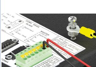
**Danger!** This device is only permitted to be supplied by a SELV / PELV (class 2) power supply or with safety extra-low voltage (SELV) in accordance with EN 60950.
