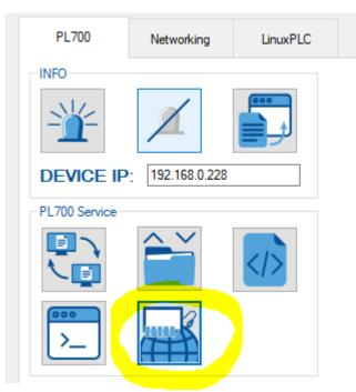
in other cases, open a Web browser and enter in the address bar, the address of the PLC specifying port 8080, for example *192.168.099:8080*
