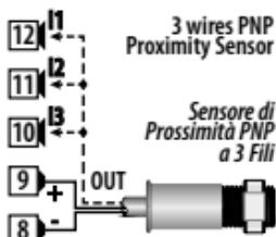
Example of connection of a 3-wires proximity sensor.
