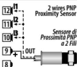
Example of connection of a 2-wires proximity sensor.
