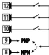
Example of connection of digital inputs in PNP and NPN mode.
