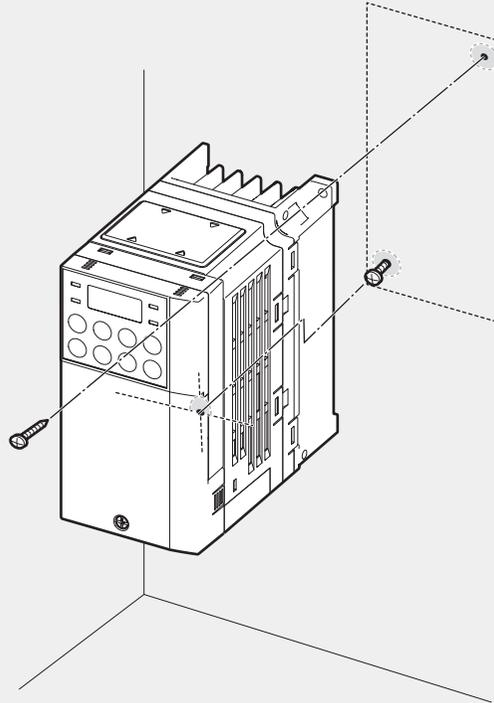
0.4-0.8kW (3-phase) inverters have only two mounting brackets.
